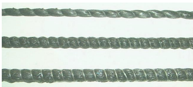
Fig. 1. Different options for creating a corrugated surface for BPR based on the use of a braid thread to create increased adhesion to concrete
